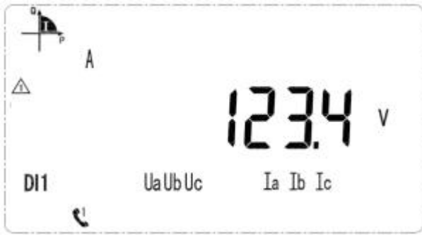
Voltage on A phase is 123.4V
