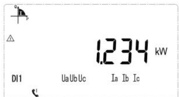
Current total power is 1.234kW
